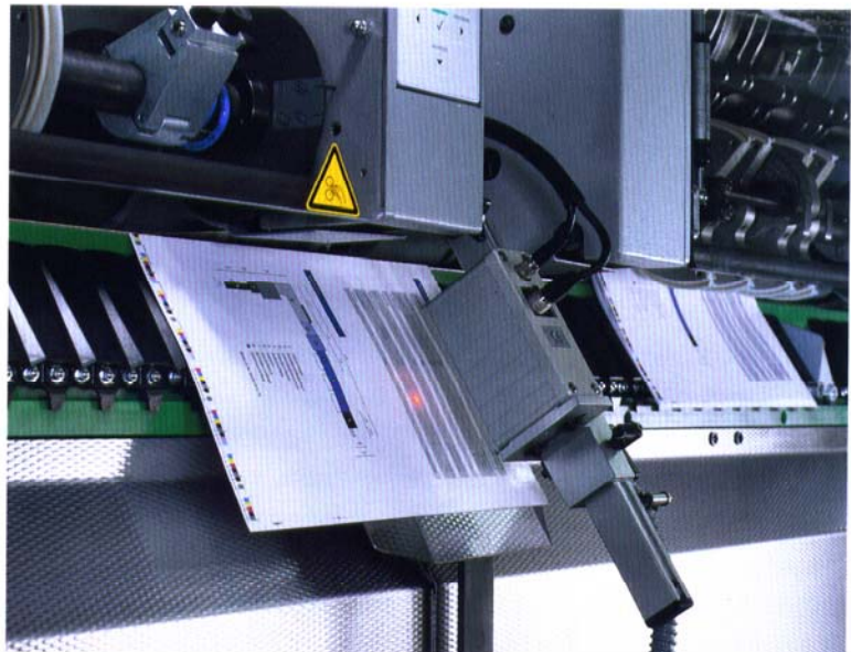
An optical camera image recognition system on the saddle chain checks signatures for correctness and make ready sheets.
