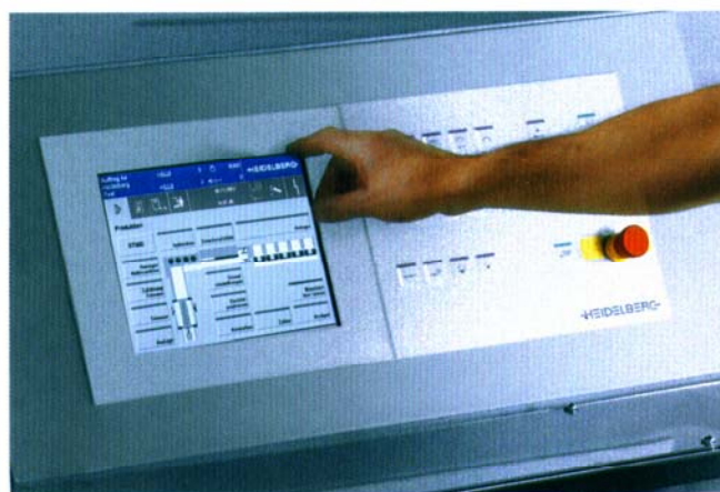
The ST 400 is monitored and operated via the touch screen control unit.
