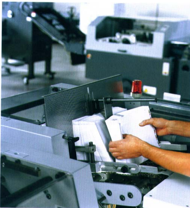
Greater flexibility than ever: position the feeder on the back side of the saddle chain.
