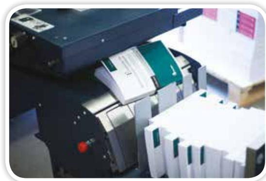
C.P. Bourg BB3002 Perfect Binder presents an efficient and an economical means of producing bound books in a wide range of sizes on-demand, with up to 13 positive or negative knife creases. The BB3002 is available in EVA/hot melt and PUR-C.
